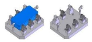
Figure 1 Typical fixture with workpiece
