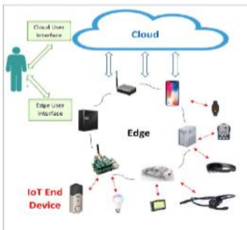
Fig.1:edge-centric computing architecture
