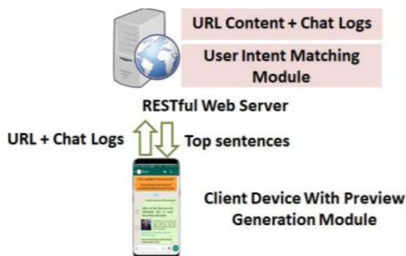
Figure 2. High level architecture of the web service to generate dynamic user previews on the mobile device.
