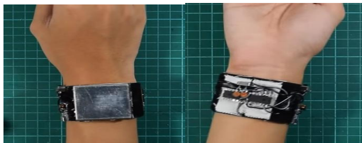
Fig Nano Version of the System fitted in a Watch like Band
