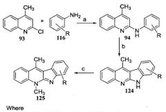
116b) R = H, 116e)R = o-Me, 116f) R = p-Me, a) Dry ethanol, reflux, 12h; b) hv, C<sub>6</sub>H<sub>6</sub>:CH<sub>3</sub>OH: H<sub>2</sub>SO<sub>4</sub>, (60:30:0.5), I<sub>2</sub>, rt; c) Me<sub>2</sub>SO<sub>4</sub>, toluene, reflux, 6 h, K<sub>2</sub>CO<sub>3</sub>, 81-82%
