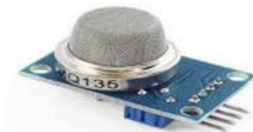
Figure 3: Air quality sensor (MQ135) for detecting a wide range of gases, including NH 3 , NO x , alcohol, benzene, smoke and CO 2
