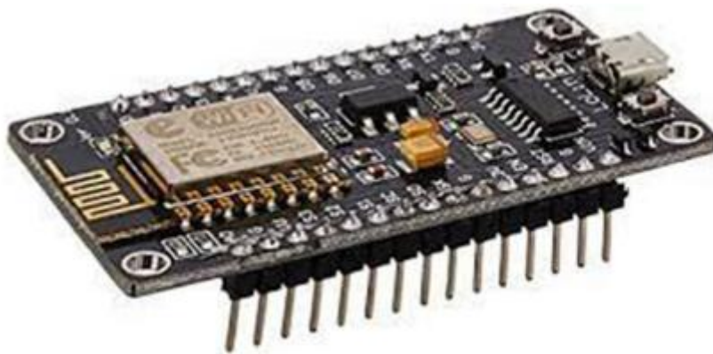
Figure 4: NODE MCU with its pin configuration
