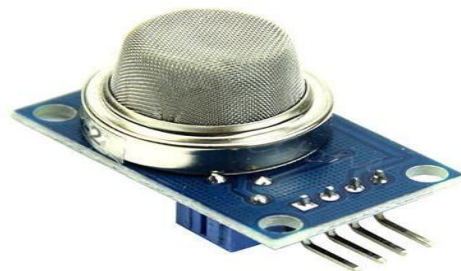
Fig.8 MQ gas sensor
