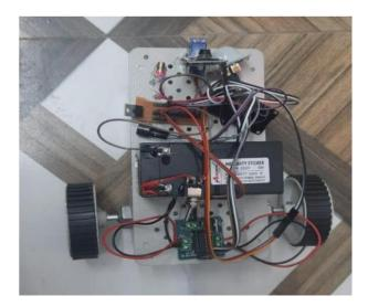
This is the spy robot which has 2 wheels at the back side which are connected to the DC motors, and one rotatable wheel at the front. The Camera, PIR sensor, Laser are connected at the front.
