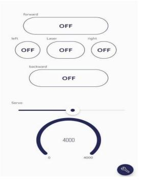
This is the page in the app when no suspicious one is detected. Through the app we can move the robot forward, backward, right and left. Also, we can move the camera around by using the blynk app.
