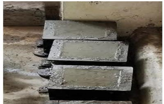
Fig. 7: Concrete block Cube mould
