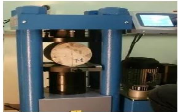
Fig.4 Compressive Strength Machine
