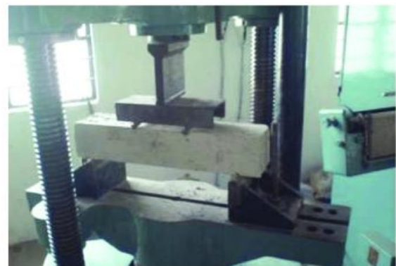
Fig.5 Flexural Strength Machine
