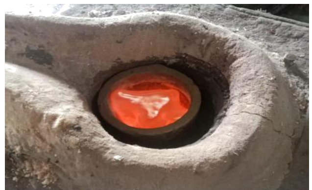
During Stir casting process
