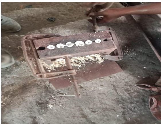
Poured composite in the mould cavity
