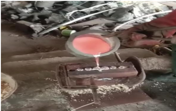
Pouring molten metal in mould cavity
