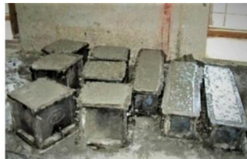
Figure 4.7 casting of samples (cubes and prisms)
