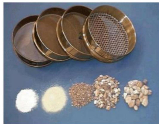
Figure 3.6 Testing fineness modulus of fine aggregates
