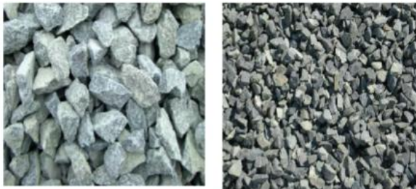
In this study coarse aggregate of nominal sizes of 20mm, 12mm are used
