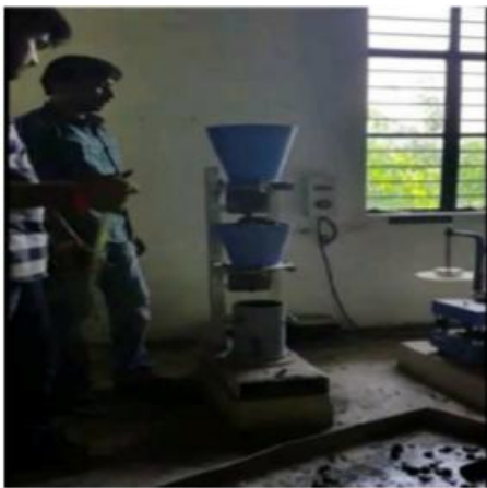
Figure 4.6 Compaction factor test
