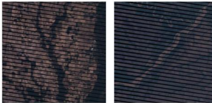
FIGURE 1. Adapted from [3]. Examples of areas having banding problems in Landsat-7 images.
