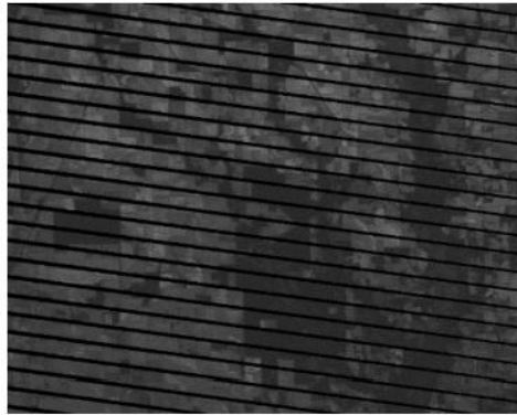
FIGURE 4. Taken from [3]. Evidence of banding in one of the spectral bands.
